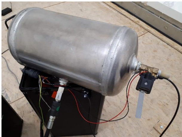
Pulse 201 (20L) unit, 1/4" air release valve. Aluminium tank not encased.
