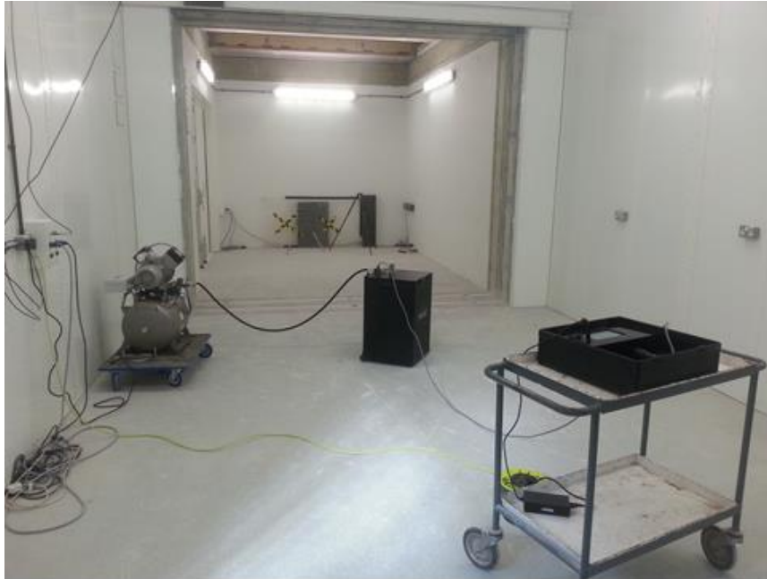
Figure 5 Chamber B - 269 m 3 Volume. Pulse set-up
