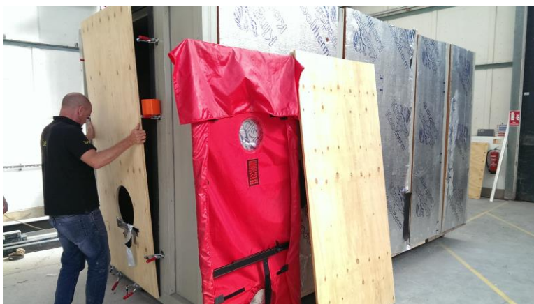
Figure 1 Chamber A, 15.98 m 3 volume. Timber panel construction, externally insulated
