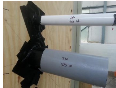
Panel B T6 (White blocked grey open) and T7 (both open) – 1 x 50mm, 1 x 110mm pipes
