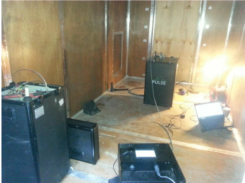
Figure 3 Chamber A – Pulse set-up inside chamber A (60L and 40L unit)
