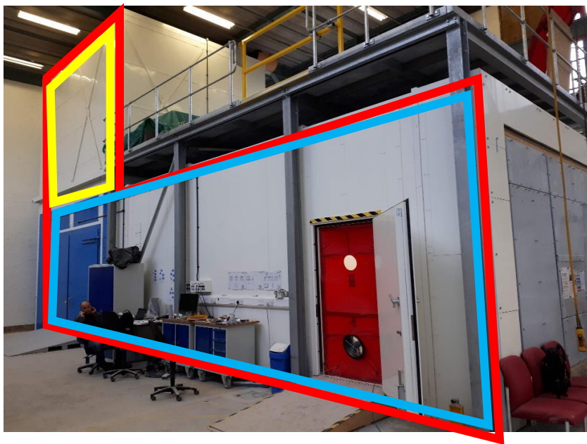
Figure 4 – External of B, C and D chamber. Red outline chamber B, blue outline chamber C and yellow outline chamber D. Solid cast concrete construction, removable timber floor cassette dividing chamber C and D.
