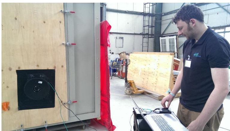
Figure 2 Chamber A – Blower Door set-up. To eradicate leakage around the door canvas and ensure like for like comparison, a ply board was used for mounting the fan in this chamber.
