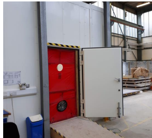
Energy Conservatory Duct Blaster and DG1000 gauge used for all chamber testing
